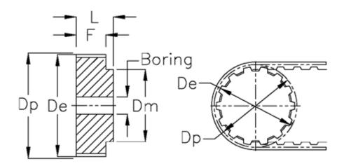
Type = AT5Belt width = - 16 mm Weight = 0.43= 94.25De Dm = 65 = 95.5 Dp F = 21 L = 27 Pre-drilled = 8 Tooth number = 60
